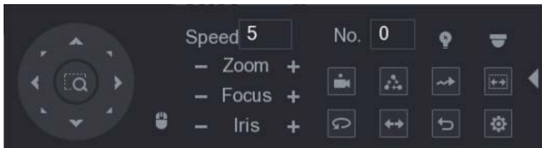
Figure 5-53 Expanded PTZ control panel
