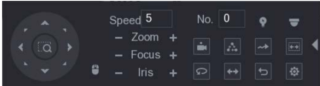
Figure 5-59 Expanded PTZ control panel
